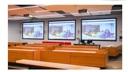
A Dalen Top-Tec Contor Duet lectern was positioned to the front of the room, this also housed all of the equipment along with a Wolfvison visuliser and wireless casting by Mersive Solstice units.
